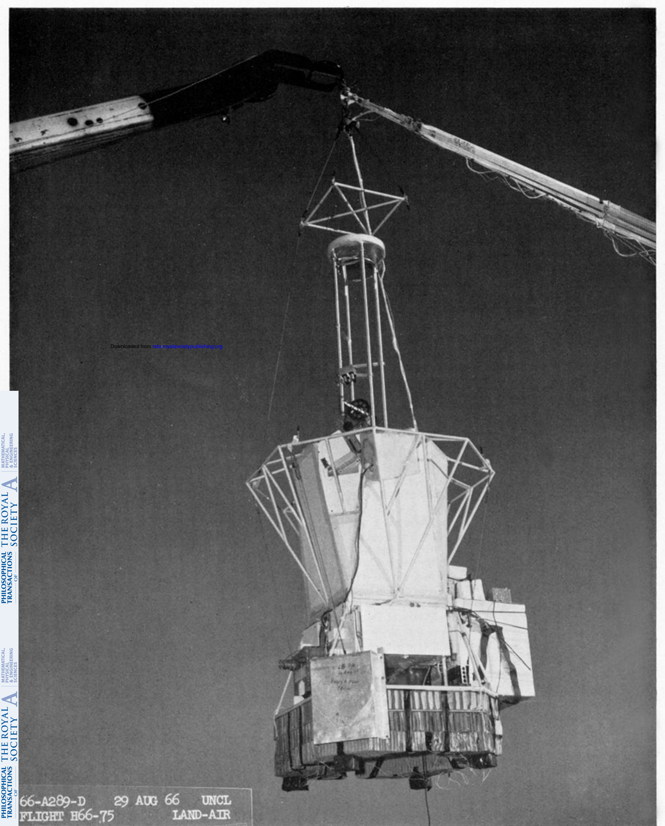
FIGURE 2. Photograph of the balloon payload in flight configuration.
